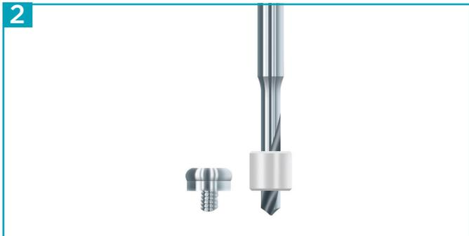
2 Hold the Cast-To LOCATOR Abutment next to the Pilot Drill and set the plastic Depth Reference Ring on the Pilot Drill to a depth that slightly exceeds the Cast-To Coping thread length.
