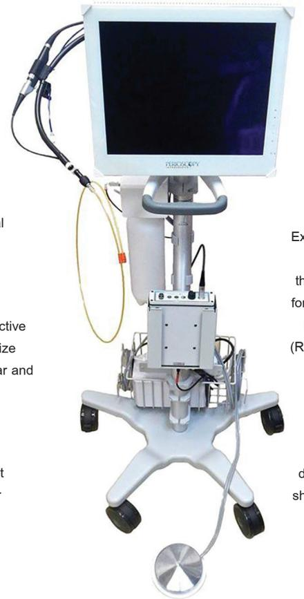
The CCD/LED camera attaches to the controller which has a focus knob for the camera and provides white balance, gain control and illumination settings.
