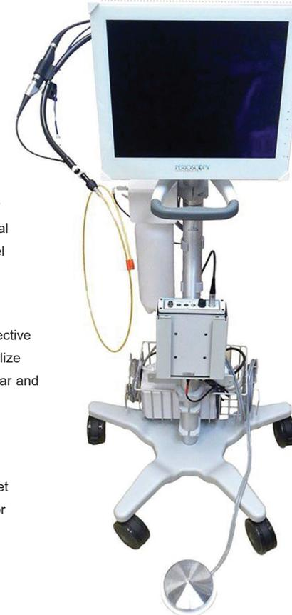
The CCD/LED camera attaches to the controller which has a focus knob for the camera and provides white balance, gain control and illumination settings.
