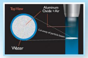
Water spray surrounds aluminum oxide to control powder spray - just like a shower curtain. Dry cutting without the mess.
