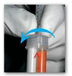
5 This photo shows the VPS material just at the mixing tip without entering it. The tab has been rotated 90° to the position above "∧" (Chevron). Material can be stored in this potion, the plunger will not extrude the material if it is inadvertently pushed.
