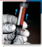
Allowing just enough empty space at the top to accommodate the plungers, the twin plungers are firmly seated into the rear of the syringe. Be careful not to push material into the mixing chamber.
