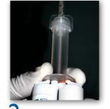
The supply cartridge, whether 25, 50, or 75ml, is firmly butted into the barrels so that there is a tight fit at the base of the syringe.
