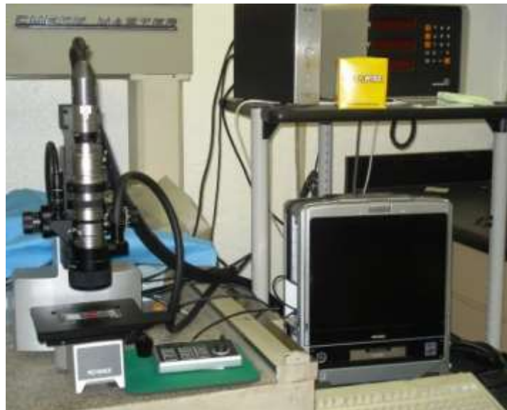
Fig 5. Keyence digital microscope VHX 600 Series
